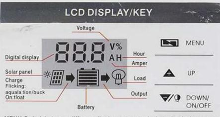
MENU: Switch between different display or to enter/exit setting by long press. :press to increaae value.
