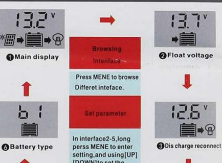
[DOWN] to set the parameter, long press MENE again to exit long press[DOWN] to restore parametet.
